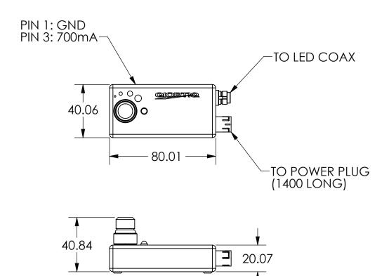
NOTE: CONTROLLER FOR 35-07-41 AND 35-07-50 ARE NOT INTERCHANGEABLE.
