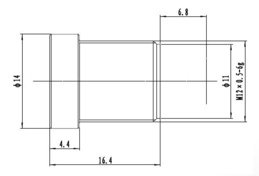
The S-Mount lens Lensagon B5M8020 is suitable for common sensors up to 5 megapixel with an image format of 1/2.5 inch. It is characterized by a particularly high light intensity.
